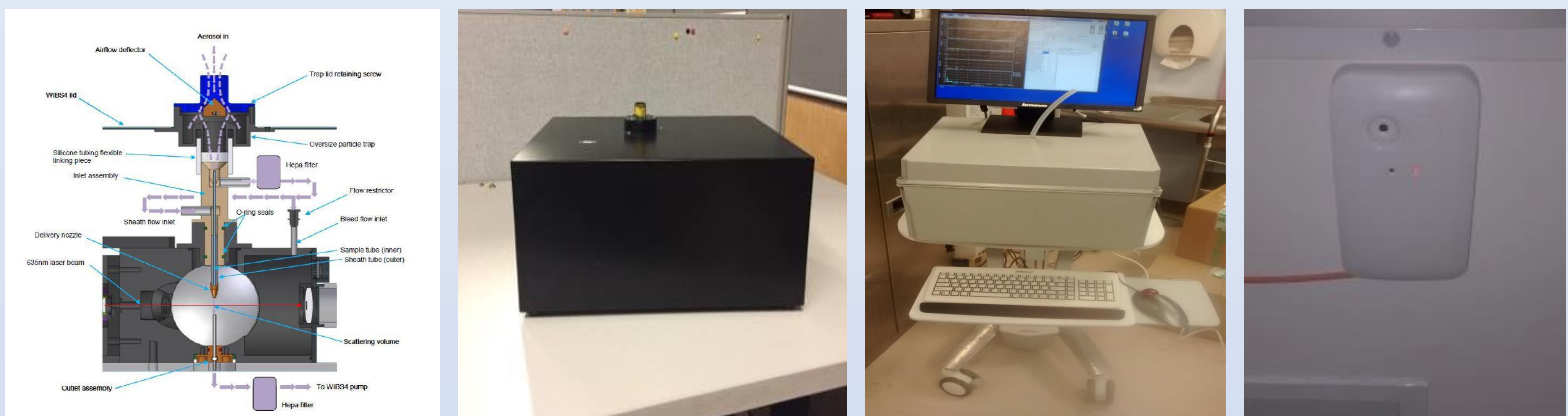
Fig 1.2 (Left) WIBS 4+ Aerosol Flow; (Middle Left) WIBS 4+ ; (Middle Right) WIBS-4+ in protective soundproof box for ward use; (Right) People counter positioned on ward ceiling.
